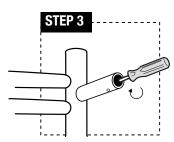
**STEP 3:** Screw down the short mounting screw (d) with a screwdriver. Note that the set screw of the tube (a) should point towards the floor when the towel warmer is wall mounted. Fix the remaining two mounting tubes (a) to the vertical bars with threaded metal pads by repeating Step 1-3.
