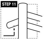
**STEP 11:** As shown in the picture, install the set screws (c) into the hole of all the tubes (a and b) using the allen wrench; fix the tube (a) onto the mounting bracket (g).
