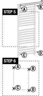
**STEP 5:** Use a tape measure to measure the distance between the center points of each wall bracket tube; record the distances between points AB, AC, CD, and BD. Mounting point C will determine electrical box location. See Electrical Assembly in following instructions.
