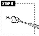
**STEP 9:** Insert long screw (i) through mounting bracket (g), then screw into plastic drywall anchor (f).
