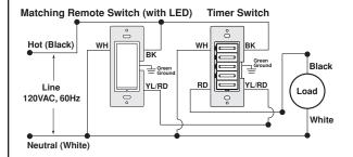
NOTE: The timer switch must be installed in a wall box that has a Load connection. The matching remote switch must be installed in a wall box with a Line Hot connection and a Neutral connection. A Neutral wire to the matching remote switch needs to be added as shown.
