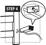
**STEP 4:** Guide the electrical cord through the electrical connection mounting tube (g) and use the long mounting screw (c) to tighten the electrical connection mounting tube to the vertical bar.
