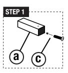
**STEP 1:** As shown in the picture, insert the short mounting screw (c) through the tube in the center of the mounting tube (a).
