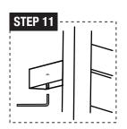
**STEP 11:** As shown in the picture, install the set screws (b) into the hole of all the tubes (a and g) using the allen wrench; fix the tube (a and g) onto the mounting bracket (e).
