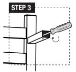
**STEP 3:** Screw down the short mounting screw (c) with a screwdriver. Note that the set screw of the tube (a) should point towards the ceiling when the towel warmer is wall mounted. Fix the remaining two mounting tubes (a) to the vertical bars with threaded metal pads by repeating Step 1-3.
