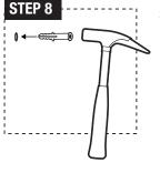
**STEP 8:** Use a hammer to knock plastic drywall anchor (d) into wall completely.
