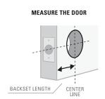
Measure distance between center of crossbore and edge of door.
