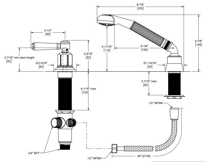
**Through-Hole Specifications** <u>Min</u> Recommended Shower: Ø1-1/4" [32] Ø1-1/4" [32] Ø1-13/16" [46] Valve: Ø1-7/16" [37] Ø 1-1/2" [38] Ø 1-3/4" [44]
