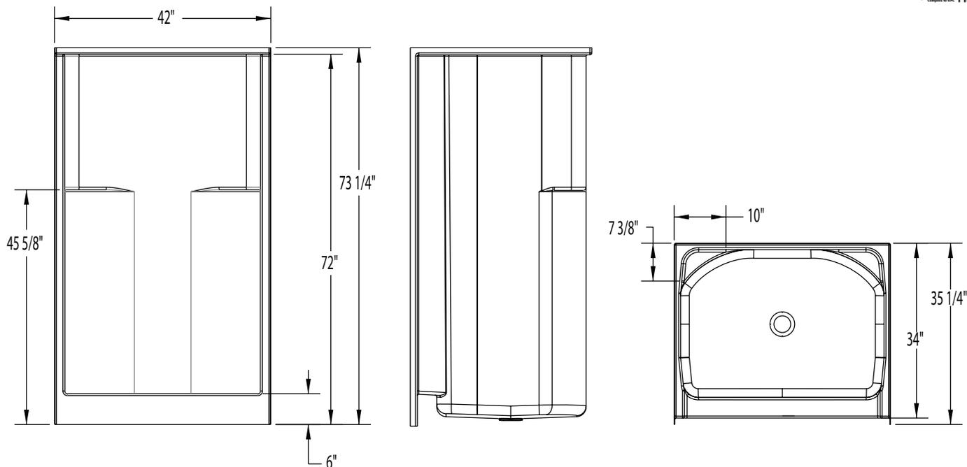
**FEATURES** lbs      Dimensional Tolerance  $\pm \frac{3}{8}$ ". Dimensions needed for site preparation should be measured from the unit. Aquatic assumes no responsibility for preparatory work.
